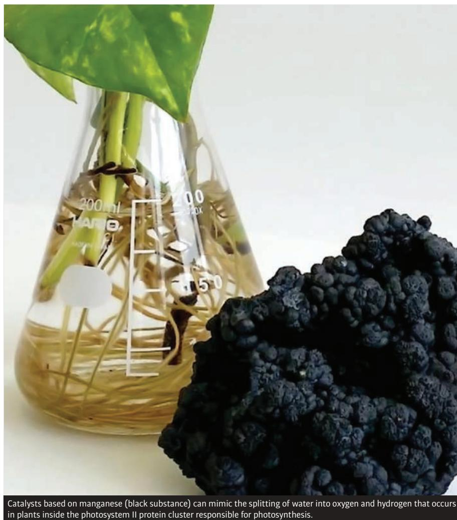
Catalysts based on manganese (black substance) can mimic the splitting of water into oxygen and hydrogen that occurs in plants inside the photosystem II protein cluster responsible for photosynthesis.
