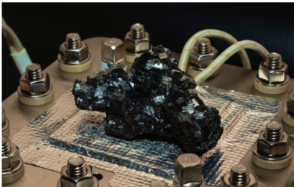
A water electrolyzer with a proton exchange membrane (PEM). The PEM contains a longer-lasting, Earth-abundant catalyst based on manganese oxide.
